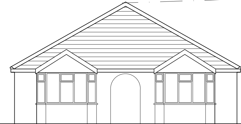
EXISTING FRONT ELEVATION
